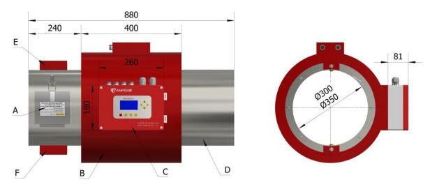
A Observation window B Metal detector C Control box D Stainless steel pipe E Spark detector SD1 F Spark detector SD2
