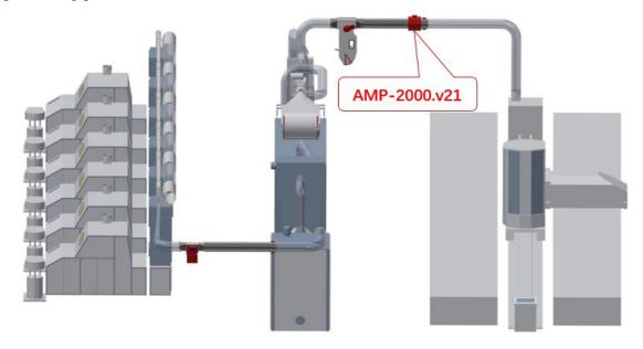
Figure 1. The installation of AMP-2000.v21 on the blowing-carding line
