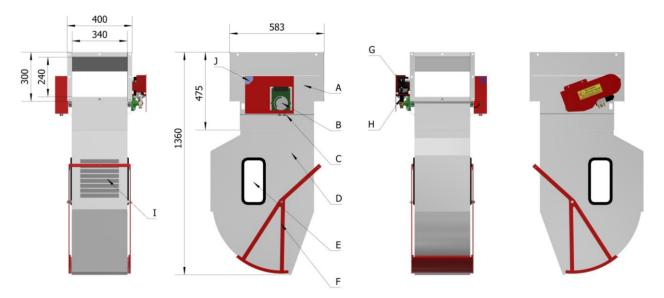
A Diverter B Display of action time C Aviation plug D Collector box E Observation window F Draw-bar G Solenoid value H Cylinder I Air supplement board J Working station indicator
