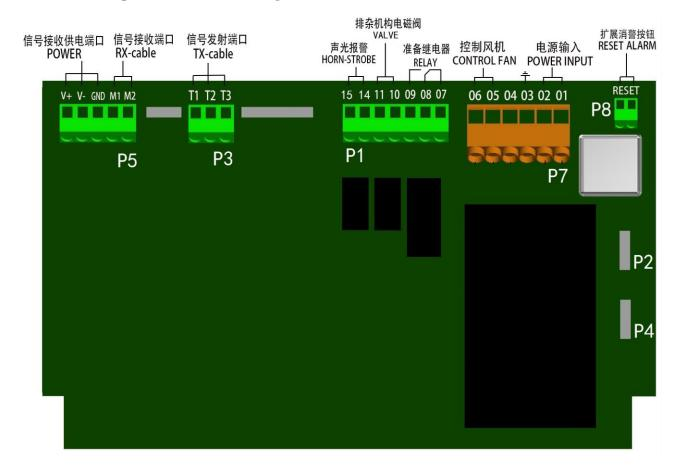
Figure 7. Wiring description of main board
