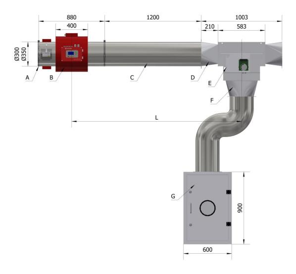
A Clamp B Metal detector C Pipe D Square to circular E Diverter F Square to circular 2
