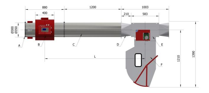
A Clamp B Metal detector C Pipe D Square to circular E Diverter F Collector box Figure 5. The stardrad installation of AMP-2000(negative and positive pressure)
