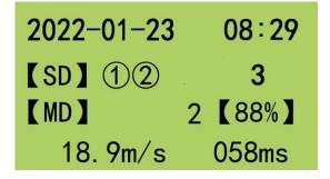
Figure 10. LCD displays content when metal alarm happpens
