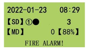
Figure 9. LCD displays content when spark alarm happpens
