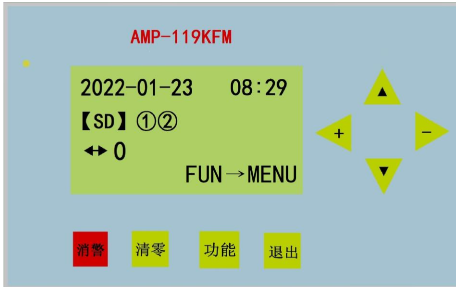
Figure 14: Operation Panel and Main Working State
